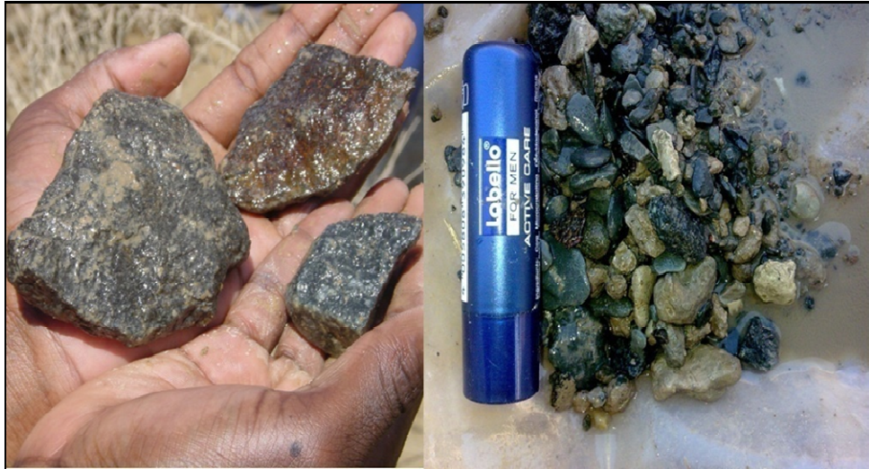
Figure 4-9: Gravel pebbles and boulders sampled during drilling of CYS1BH3 at a depth of 11-18 metres.
