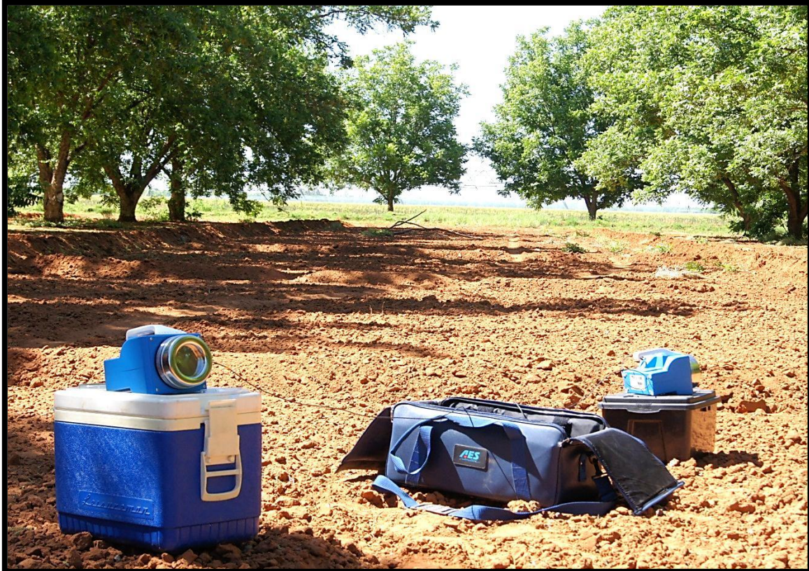
Figure 4.6: The AES air sampler setup for the collection of fungal propagules from the air at one of the selected trees in the pecan orchard (Photo by J. Saaiman).
