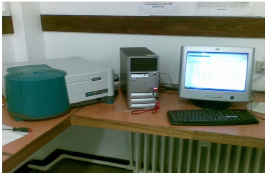
Figure 3.7: PL spectroscopy from Carry Eclipse Fluorescence Spectrophotometer System, equipped with a 150 W xenon lamp as the excitation source.
