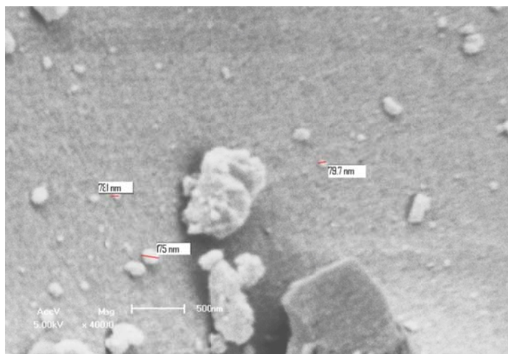
Figure 5.2: SEM images of \text{SiO}_2:0.5\% \text{Ce}^{3+} nanoparticles showing aggregation and spherical nanoparticles.
