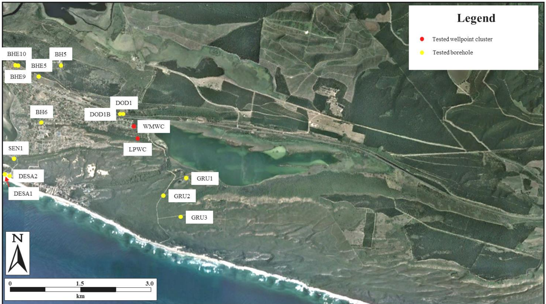
Figure 5.2: Locations of boreholes and wellpoint clusters subjected to constant discharge pumping tests.
