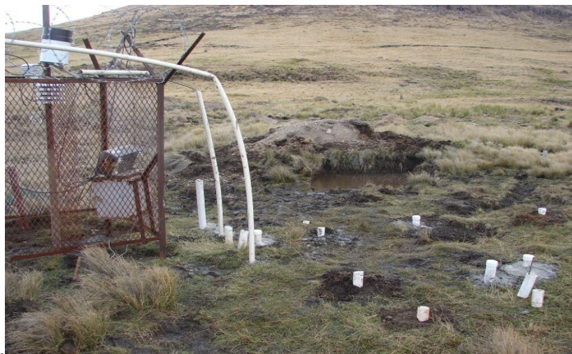
Figure 3-5 Weather station and sensors installed at Bokong in wetland PW32.
