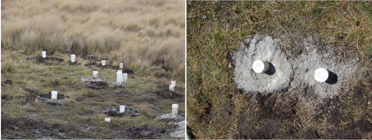
Figure 3-9 A number of installed piezometers at PW32 wetland sealed with bentonite and covered at the tops and the depth labelled on top of the caps.
