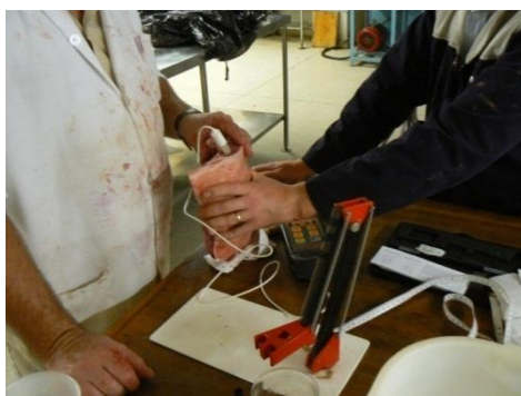
Figure 3.12 Measuring meat pH between the 12 th and 13 th rib.
