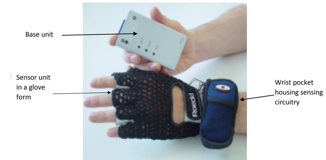
Figure 10: EREC II components
