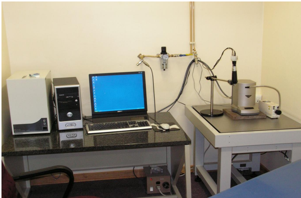
Figure 3.5. The atomic force microscopy (AFM) unit at the Physics Department, University of the Free State.
