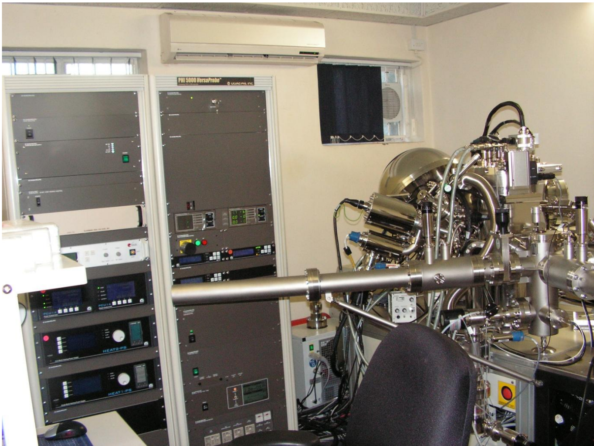
Figure 3.9. The PHI 5000 XPS Versaprobe (monochromatic AlK\alpha lines) machine at the Physics Department of the University of the Free State.
