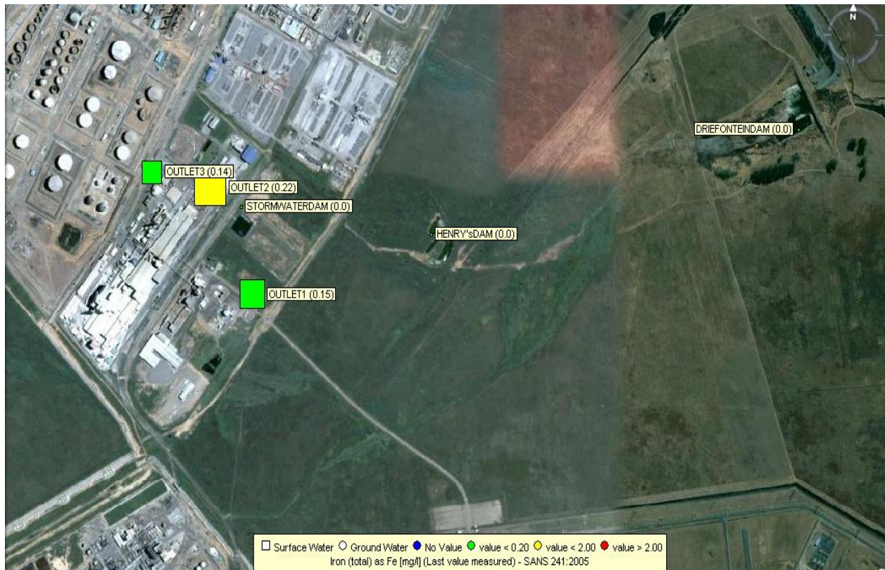
Figure 209: Iron surface water monitoring results.
