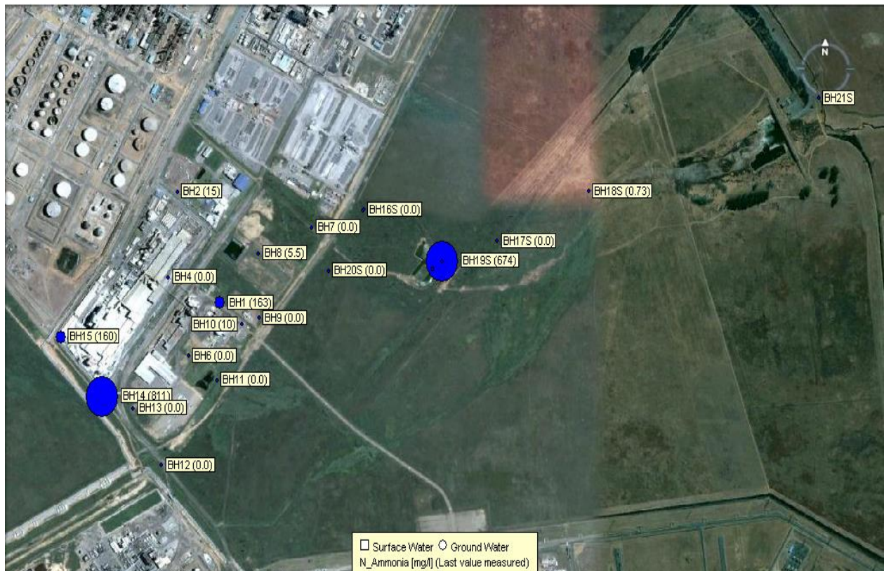
Figure 142: Ammonia last measured value shallow boreholes minus background water quality SANS 241:2006.
