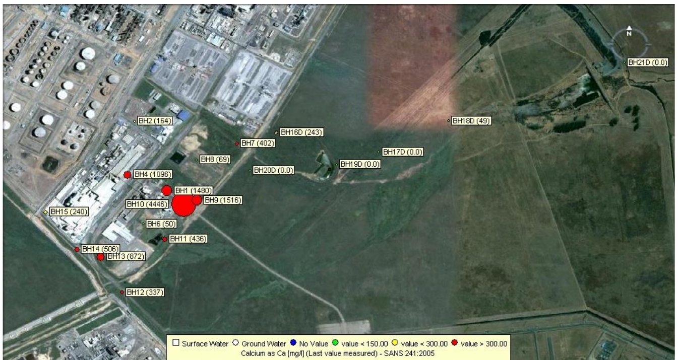
Figure 60: Calcium last measured value deep boreholes minus background water quality compared against SANS 241:2006.
