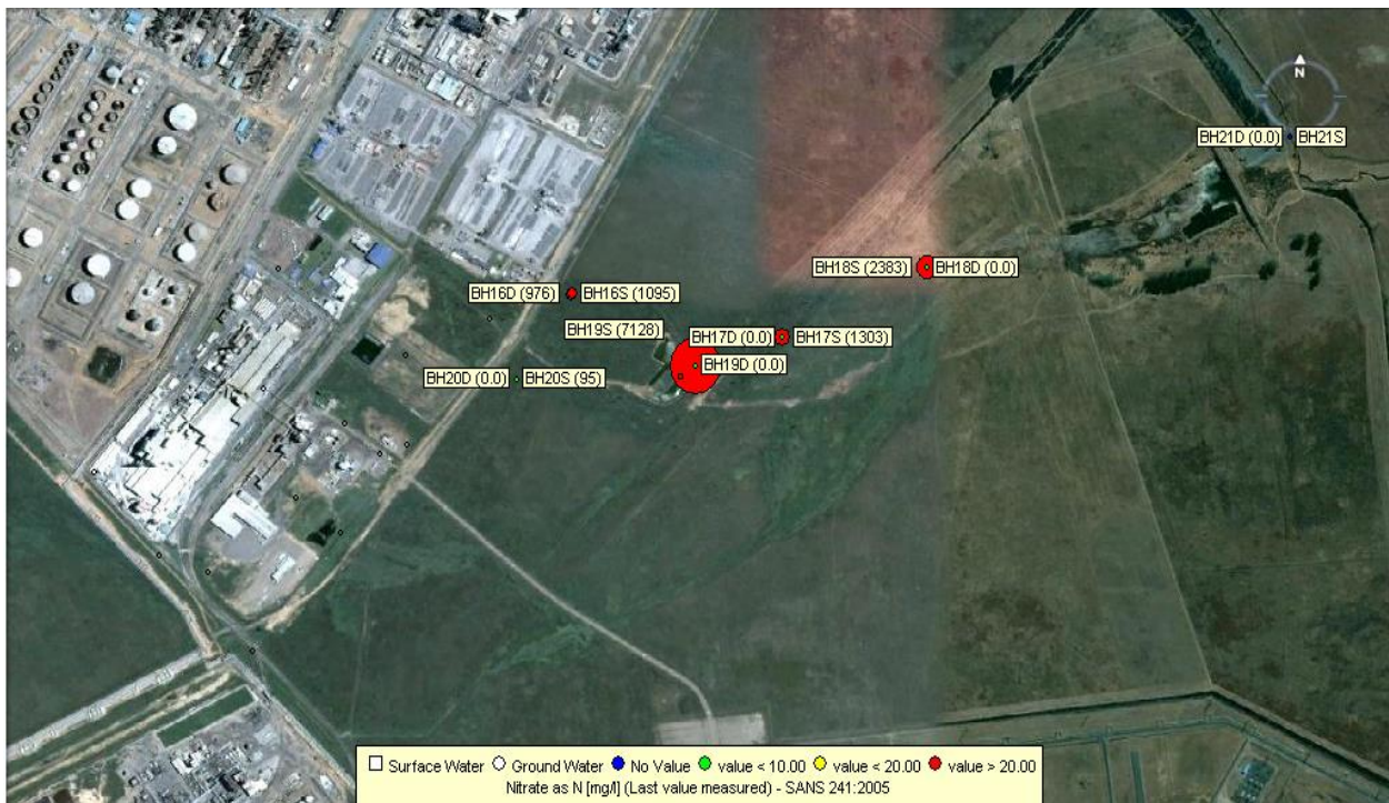
Figure 164: Nitrate last measured value shallow and deep boreholes minus background water quality SANS 241:2006.
