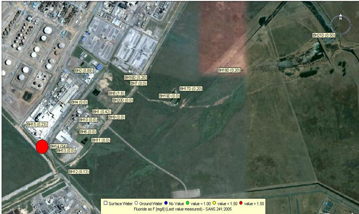
Figure 75: Fluoride last measured value deep boreholes.
