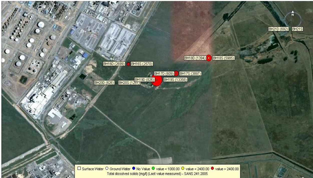
Figure 189: TDS last measured value shallow and deep boreholes comparison SANS 241:2006.
