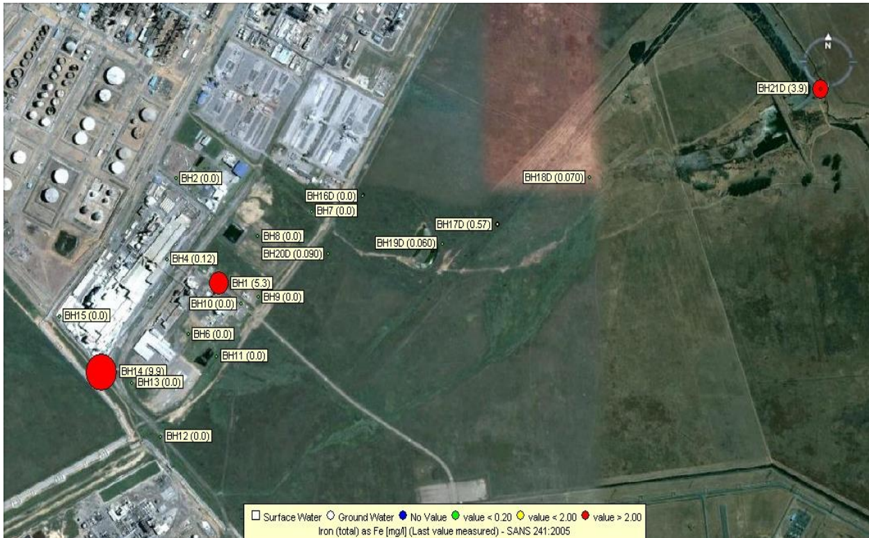
Figure 85: Iron last measured value deep boreholes.
