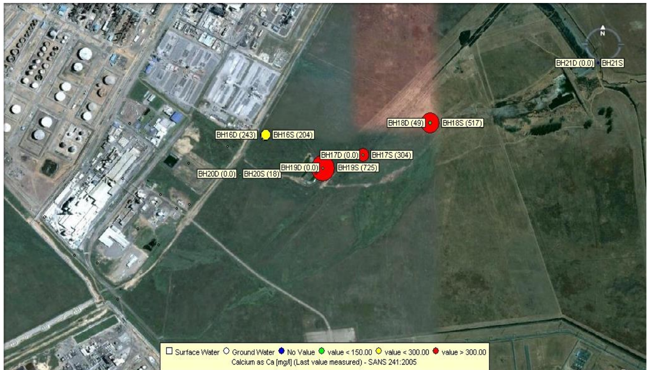
Figure 64: Calcium last measured value shallow and deep boreholes minus background water quality compared against SANS 241:2006.
