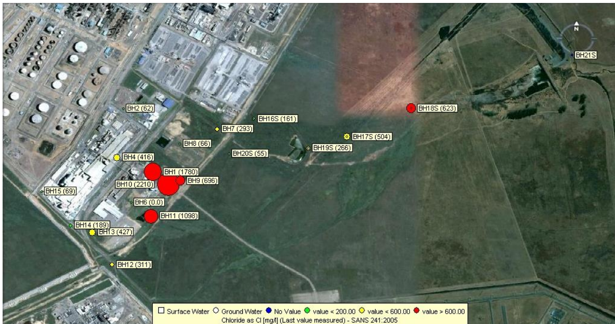
Figure 72: Chloride last measured value shallow boreholes minus background water quality compared against SANS 241:2006.
