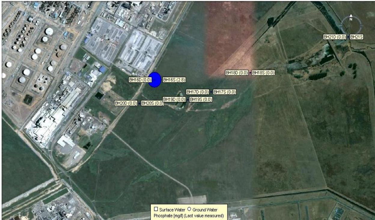
Figure 169: Phosphate last measured value shallow and deep boreholes comparison SANS 241:2006.
