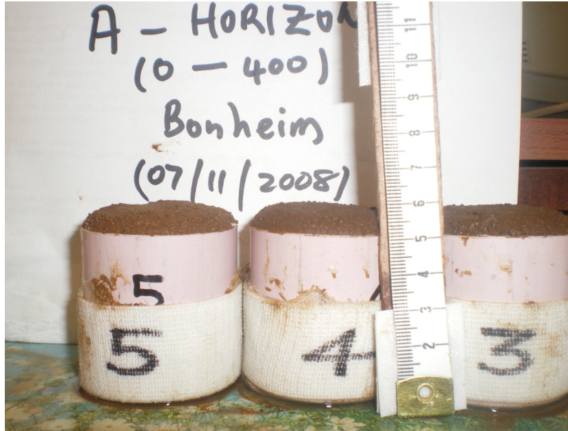
Figure A1.1 Photo showing the swelling properties of the melanic A-horizon (Section 2.2.1)
