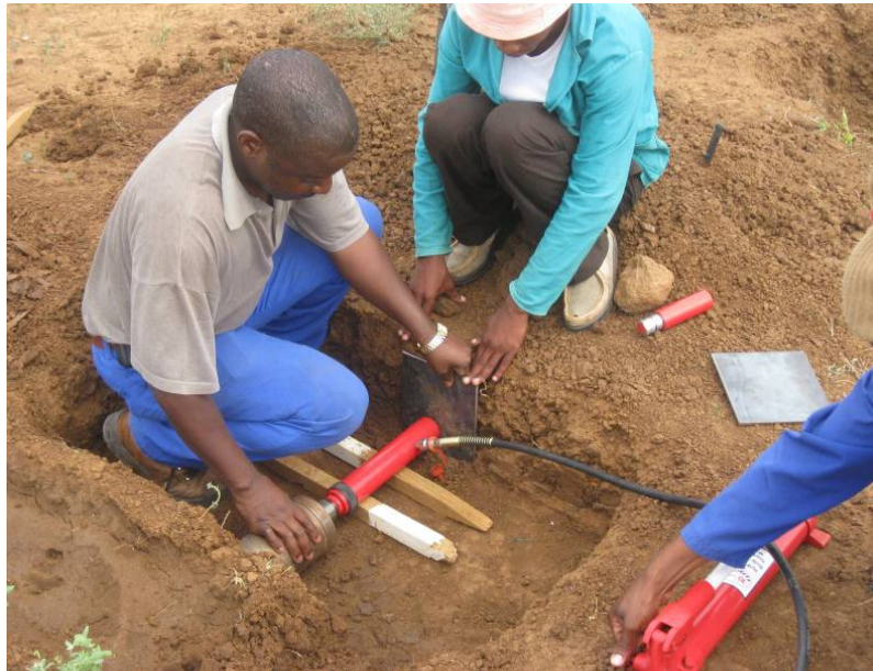
Figure 2.3 The modified hydraulic jack positioned in a profile pit of the melanic A-horizon to take undisturbed soil cores (105 mm diameter and 200 mm length).
