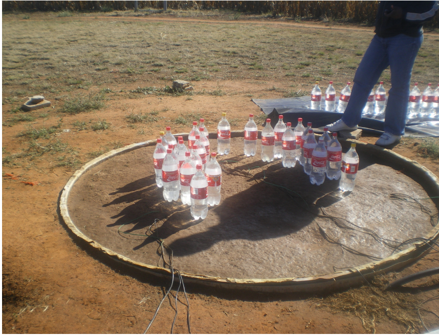
Figure A8.1 Photo showing weighing lysimeter on it, some of the two-liter bottles used for calibration
