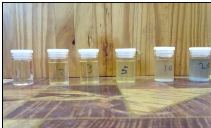
Figure 4.4: Influence of PPDA concentration on precipitation of \text{NbF}_5 and \text{TaF}_5 in ethanol ( \text{pH} = 5.10 ).
