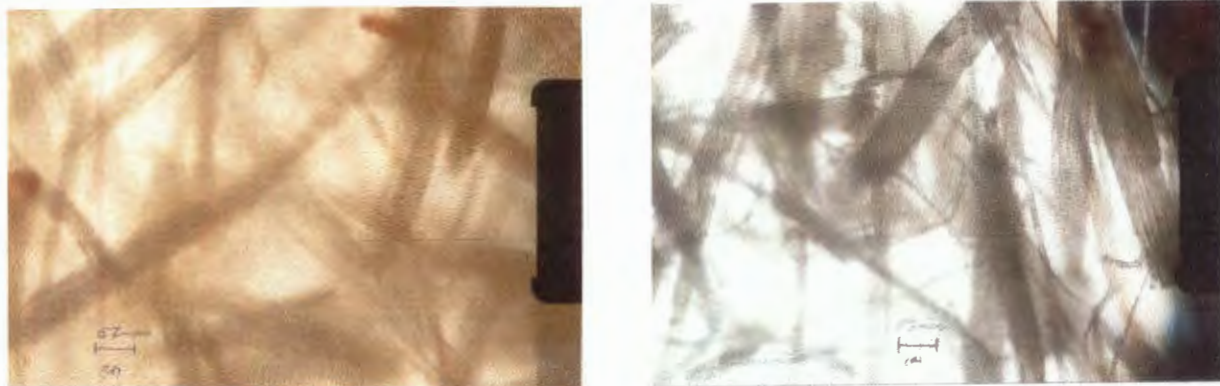
Figure 3.35 Optical microscopy photos of 77/3/20 (left) and 79/1/20 w/w LLDPE/DCP/sisal (right)
