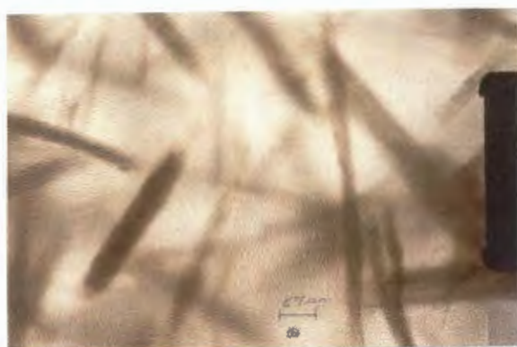
Figure 3.36 Optical microscopy photo of 87/3/20 LLDPE/DCP/sisal
