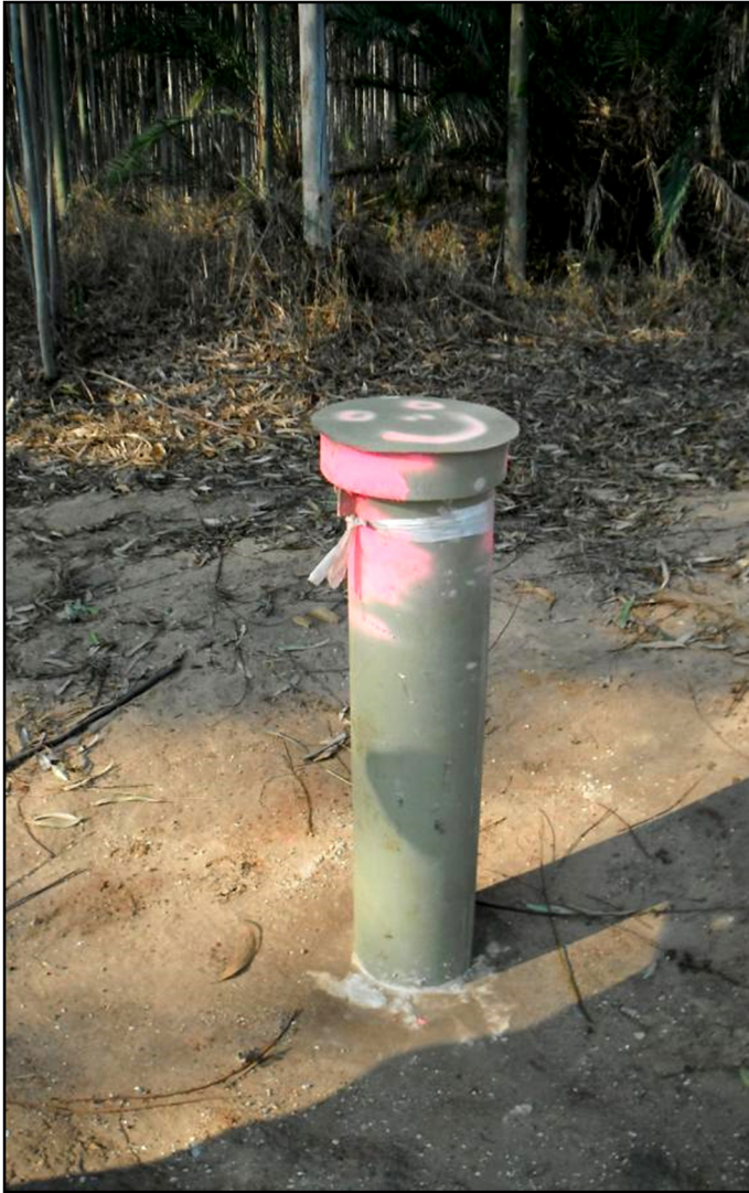
Figure 47: Monitoring borehole WES01
