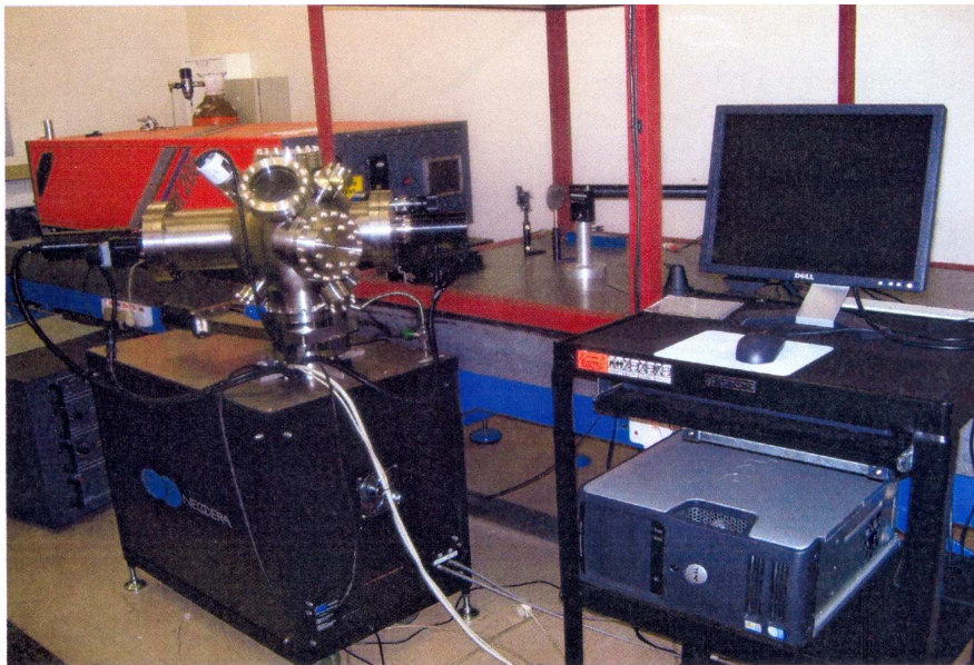
Figure 3.9: 248 nm KrF Lambda Physik excimer laser with PLD setup
