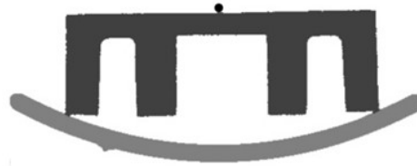
Figure 2.3. Transverse slice of the segmented CT image of the source, Styrofoam block and patient bed.
