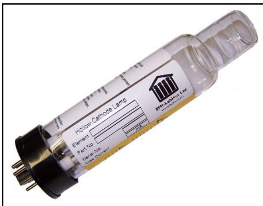
Figure 4.15: Varian coded 37mm hollow cathode lamp for Nd analysis. 148
