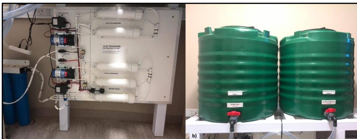
Figure 5.5: a) Ultra reverse osmosis system b) ultra-pure water storage tanks.
