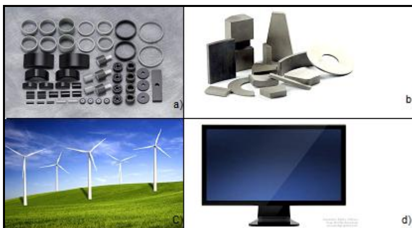
Figure 2.12: a) Neodymium-iron magnets b) samarium cobalt magnet (SmCo 5 , Sm 2 Co 17 ) c) wind turbine and d) computer screens.
