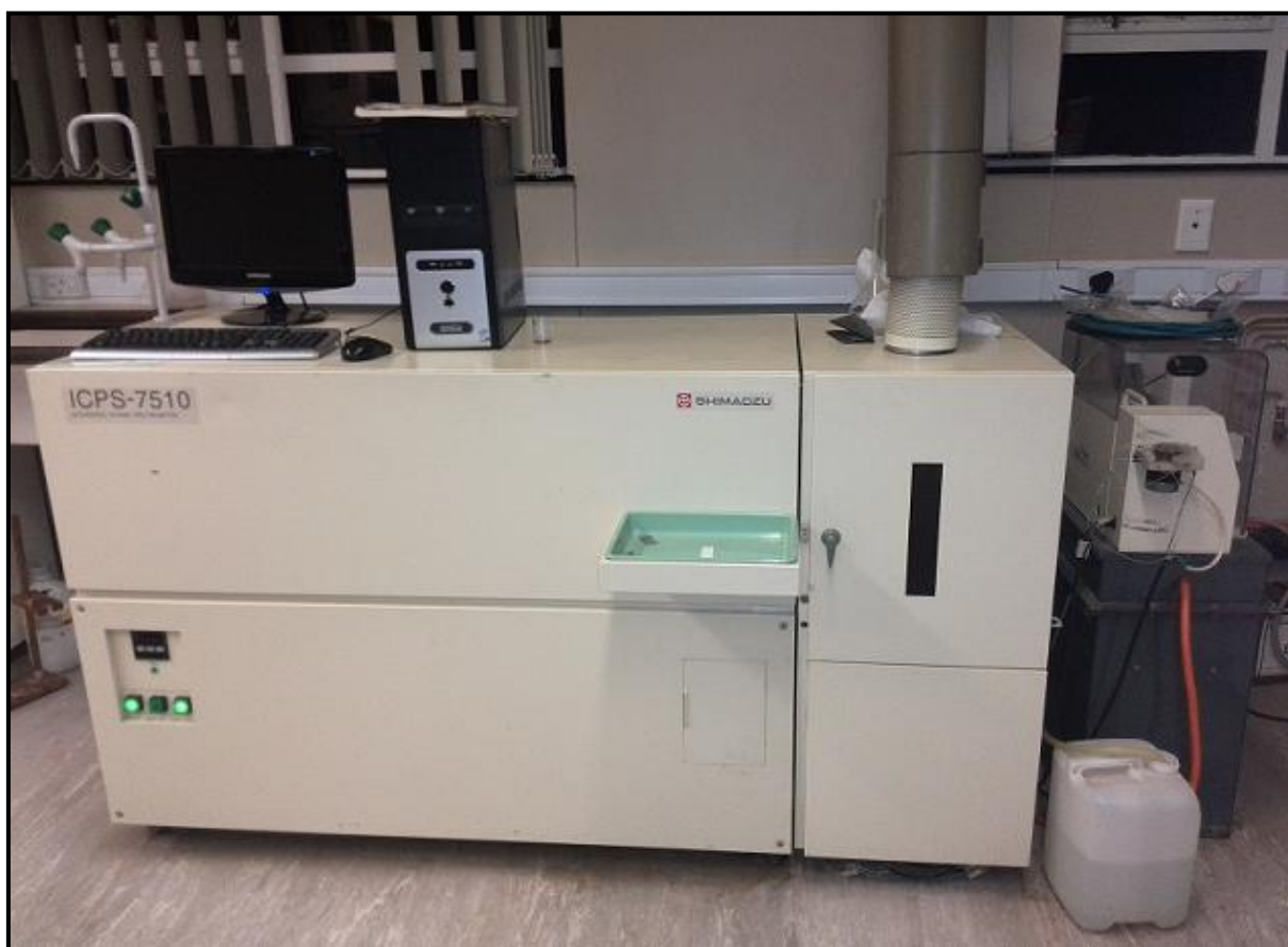
Figure 5.1: Shimadzu ICPS-7510 radial-sequential plasma spectrometer.
