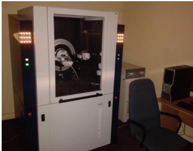
Figure 3.4 D8 Bruker Advanced AXS GmbH X-ray diffractometer at the University of the Free State
