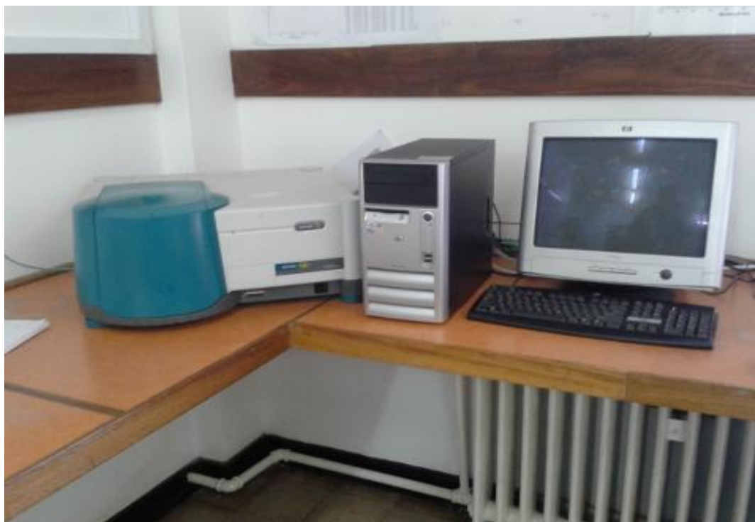
Figure 3.10 the Cary Eclipse Fluorescence Spectrophotometer at the University of the Free State, Physics Dpt.
