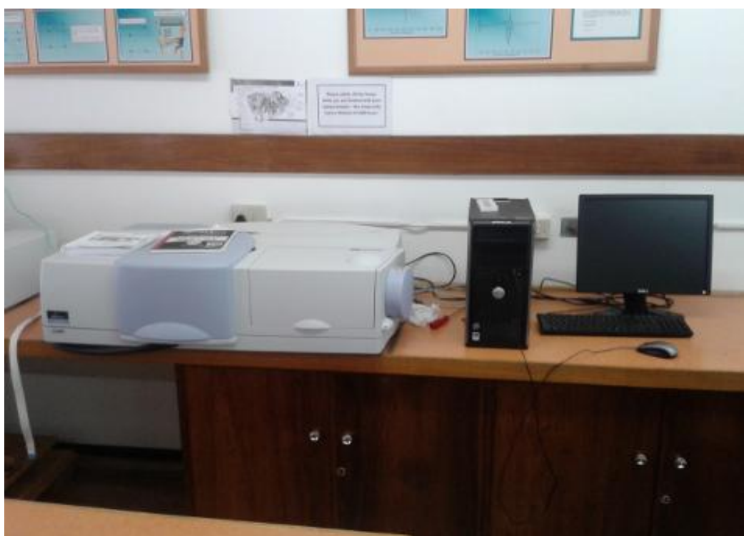
Figure 3.11 Perkin Elmer lambda 950 UV-VIS Spectrometer at the University of the Free State, Physics Department.
