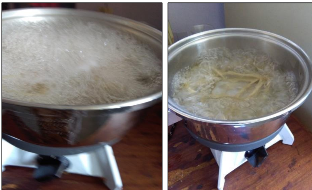
Figure 3.7: Agave americana L. fibre boiled in water as a pre-treatment process
