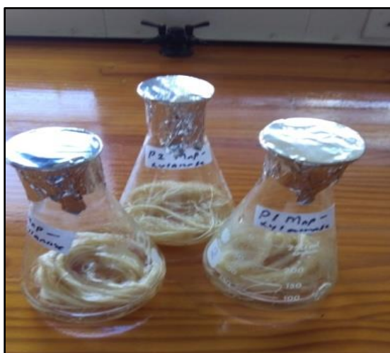
Figure 3.10: Agave americana L. fibre with enzyme solution before incubated in the convection oven
