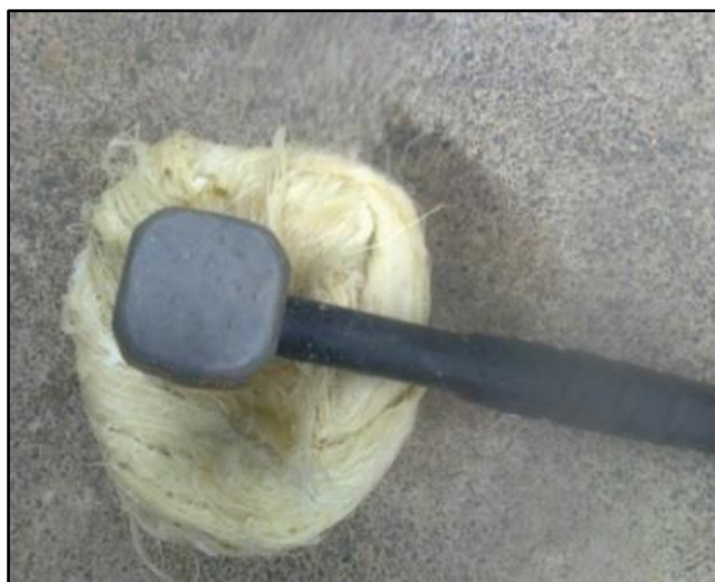
Figure 3.5: Agave americana L. fibre lightly hammered to degrade the binding components
