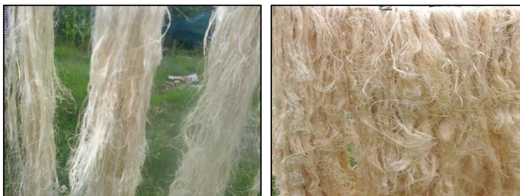
Figure 3.6: Extracted Agave americana L. fibre hung to air dry
