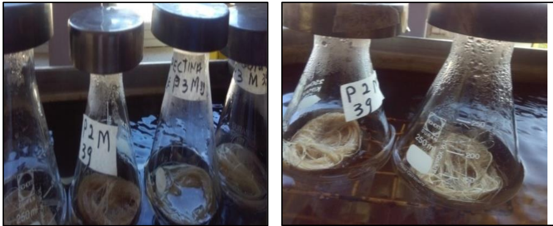
Figure 3.8: Enzymatic biosoftening of Agave americana L. fibre incubated in water bath
