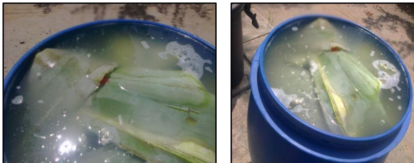
Figure 4.1: Retting process started with leaching and a gaseous fermentation
