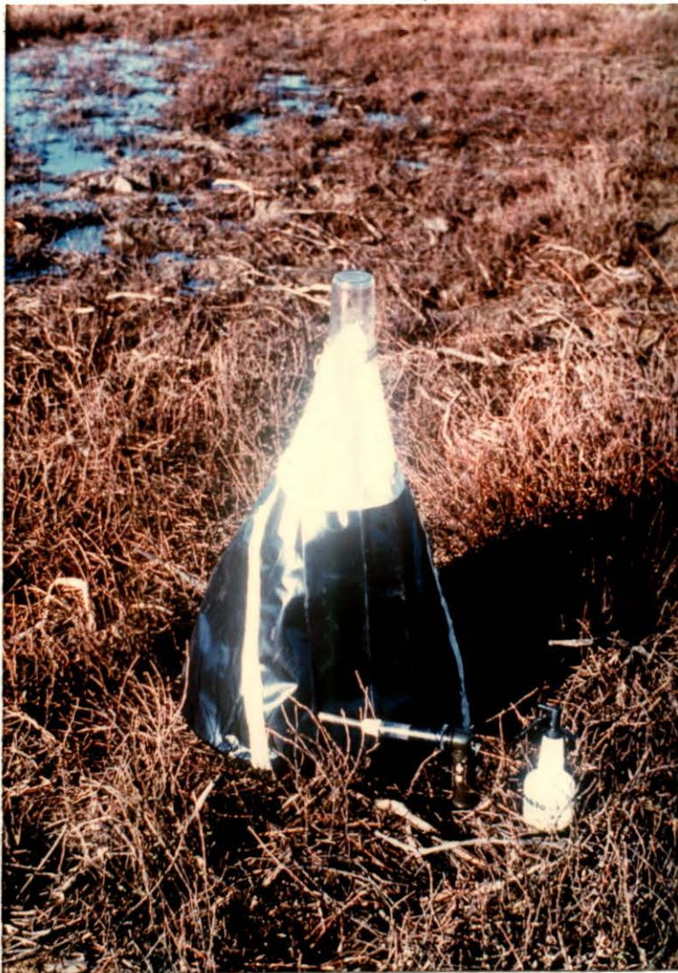
Fig. 2.11 The mosquito emergence trap used to sample adults during winter.
