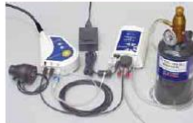
Fig. Calibration equipment and test setup for performing an automatic gas calibration.
