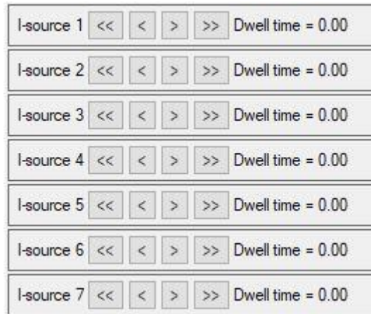
Figure 16 - Interstitial needle planning tool. The tool allows for manual dwell time adjustments of the additional 7 sources used in the IC/IS planning process.
