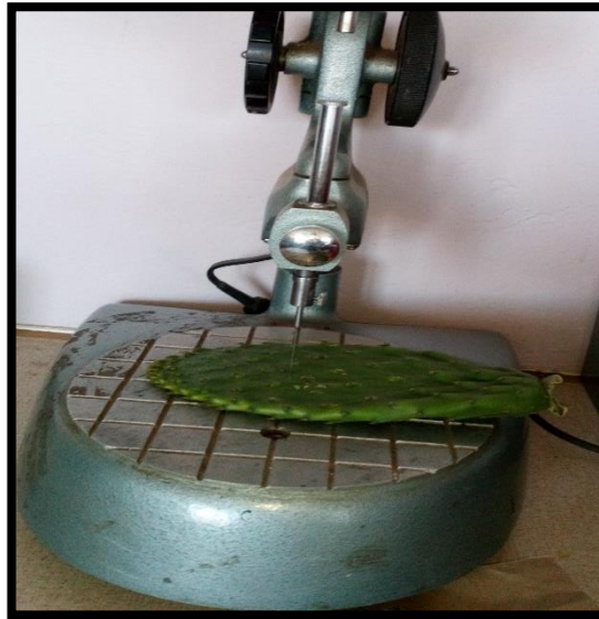
Figure 3.5: The needle of the penetrometer penetrating through the young cladode
