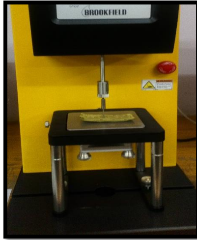
Figure 5.7: A sample placed on the fixture base table of a texture analyser
