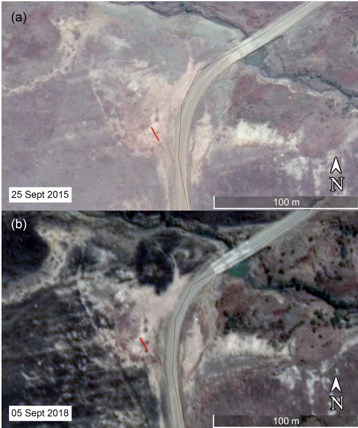
Fig. S4.2: Sattelite images of Site A on (a) 25 September 2015 and (b) 5 September 2018 showing further erosion over time. Images obtained from Google Earth 7.3.2.5776. Viewed 24 March 2020. Red line indicates position of the rock-wall gabion.
