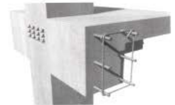
Fig: Detail 2: Slab, beam, column connection Sourcebimandbeam.typepad.com
