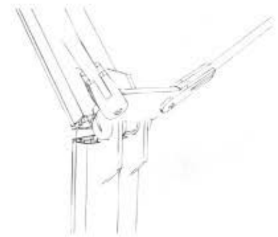
Fig: Steel cable connection, holds EFTE membrane in suspension
