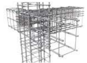
Fig: Reinforcement detail of slab, beam and column connection Sourcebimandbeam.typepad.com
