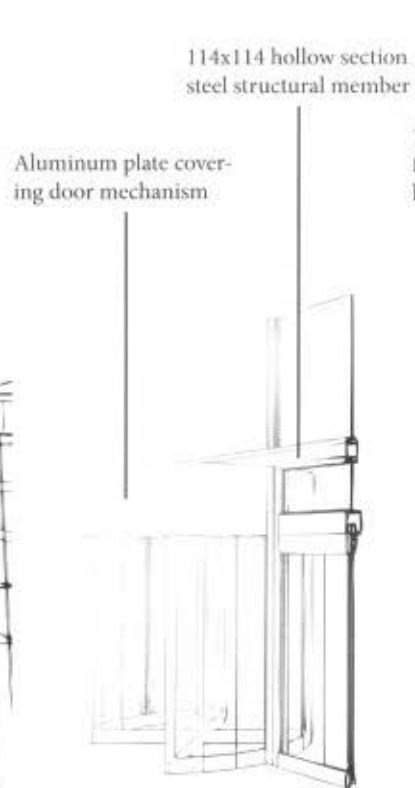
Fig: 3D Section drawing of aluminum sliding door. (entrance)
