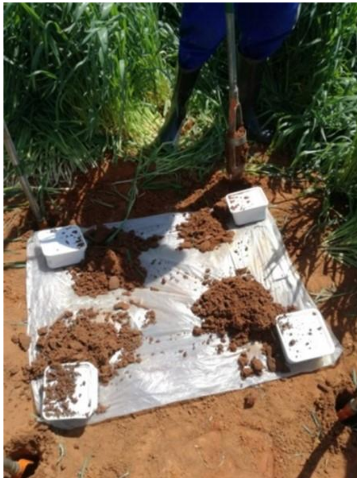
Figure 3.9 Soil samples collected from the four corners of the 1 m 2 cleared area in a selected field to prepare a composite sample.
