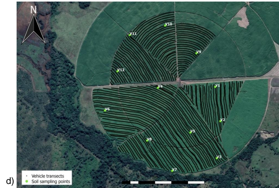
Figure 3.6 Route maps of transects driven by the mobile sensor unit showing EMI measuring points and soil sampling points at the a) Douglas, b) Luckhoff, c) Hofmeyr and d) Empangeni study sites.
