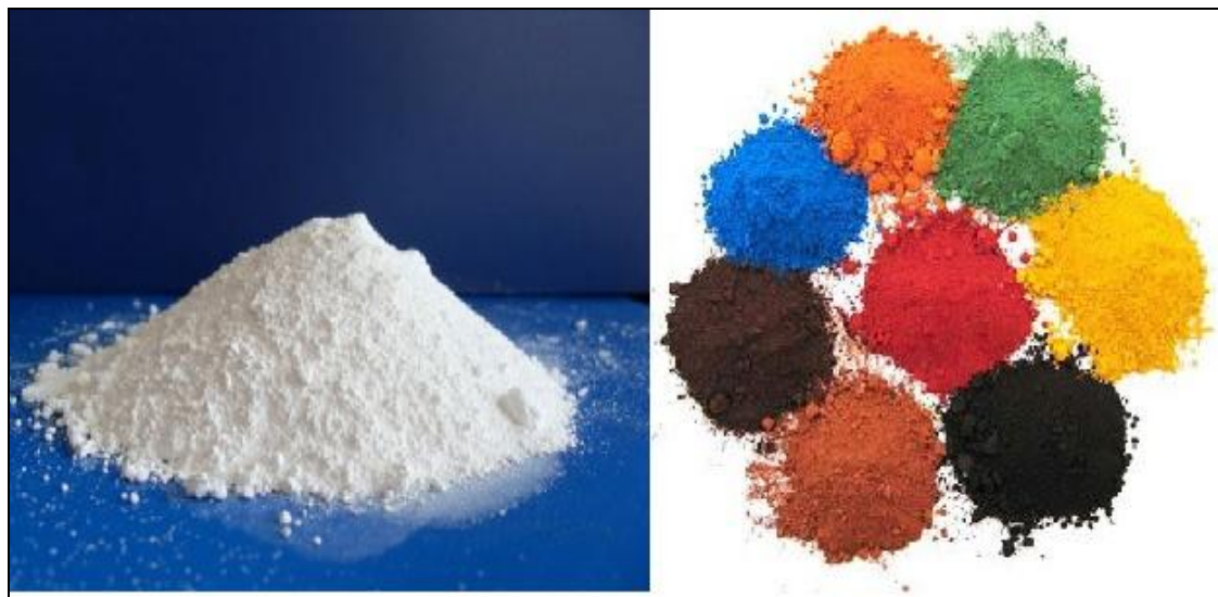
Figure 2.13: Titanium dioxide powder and iron oxide powder producing dyes with different colours. 79,80
