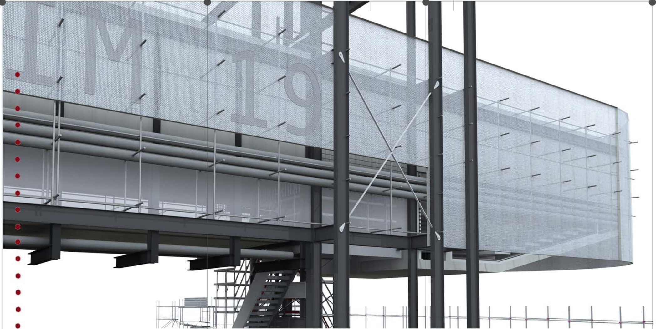
Illustration 6.46 Translucent textile membrane: the grey coloured fabric composed of glass fibre with silicone spread across two sides, is a transition and filter between the large 5 meter high foyer with its steel structure and the outside.
