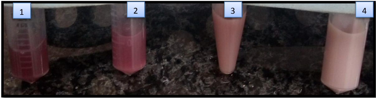
Figure 4.1a: Raw full-cream milk tested by the alizarol test for quality at varying times after treatment with KIO_3 . Tube 1; raw full-cream milk sample incubated at 5^\circ C for 48 h; Tube 2; raw full-cream milk sample incubated at 25^\circ C for 48 h; Tube 3; raw full-cream milk sample incubated at 5^\circ C for 0 h and Tube 4; raw full-cream milk sample incubated at 25^\circ C for 0 h
